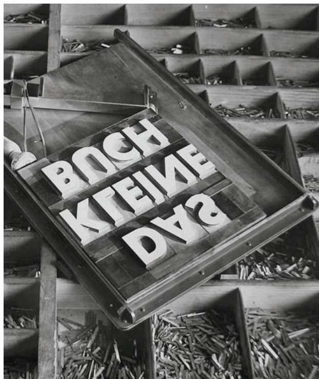
1930s technology: typecase with composing stick, punches and galley
